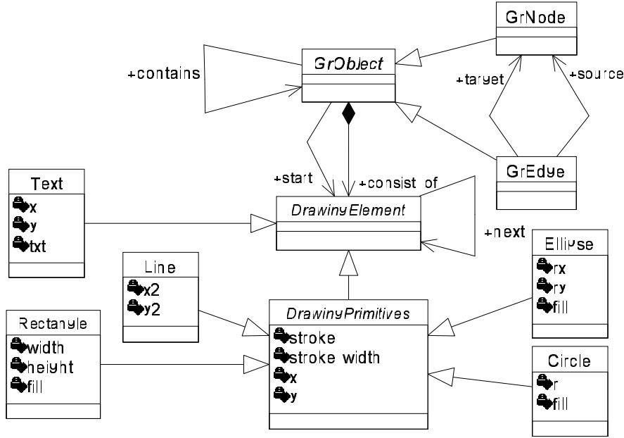
Fig. 3. An extract from the metamodel of drawing primitives
