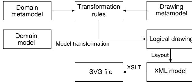
Fig. 1. An overview of the visualization process
